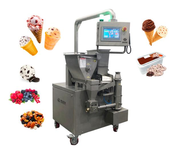
The ingredient feeder is installed between a continuous freezer and a filling machine that dispenses ice cream into consumer containers (cups, cones, tubs, etc.).
